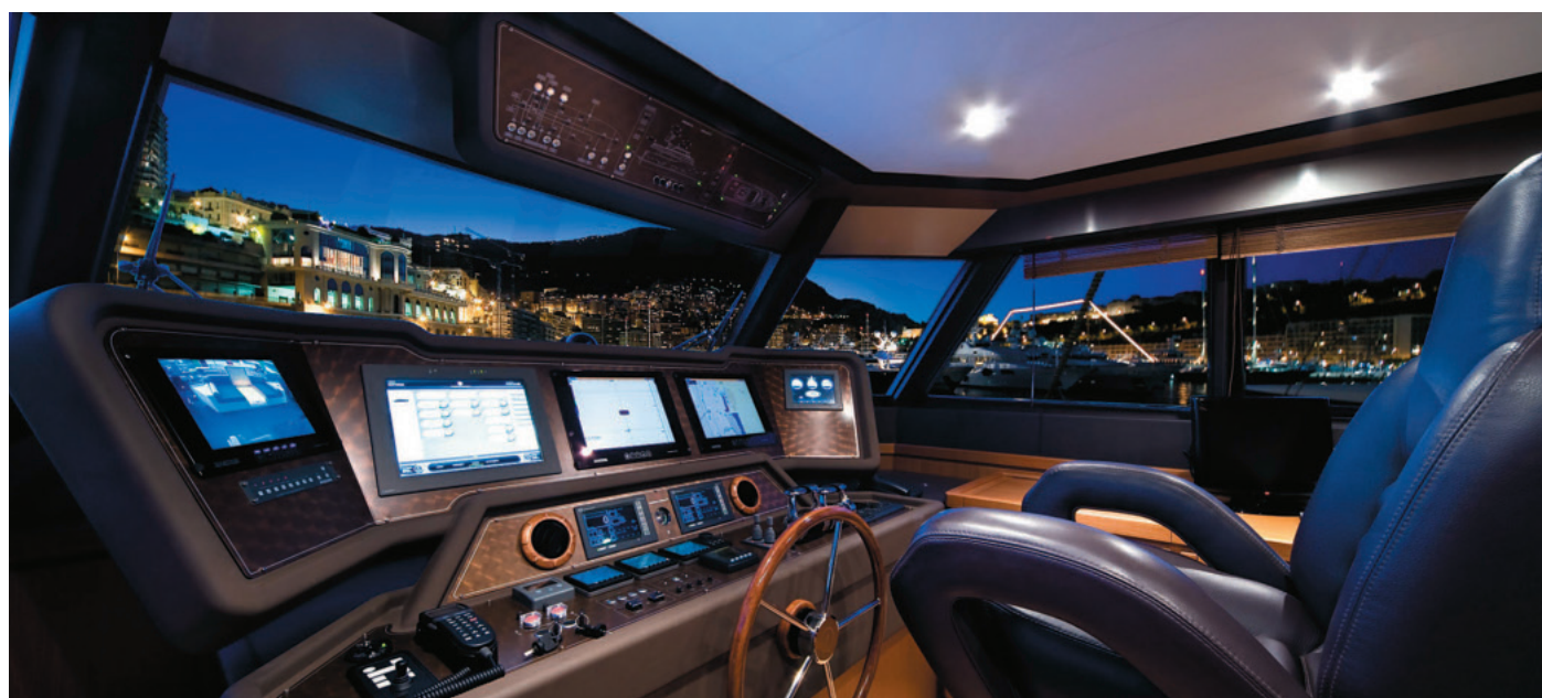
A pleasant helm station clearly displays all information; the touchscreen on the far right allows switching modes of operation
